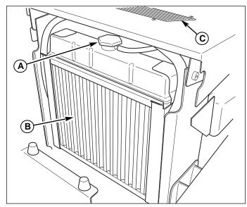
Figure 16. Radiator & Oil Cooler
